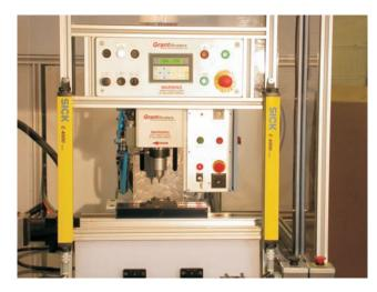
X-Y-Z riveting systems are available in 1/16", 1/8", 3/16", 1/4" semi-tubular diameter rivet capacities. For solid steel rivet diameter capacities we offer Orbital, Twin-Spin roller, and Spin-press burnishing forming technologies. X-Y-Z riveting systems are available in 3mm, 5mm, 8mm, 12mm and 16mm capacities.
